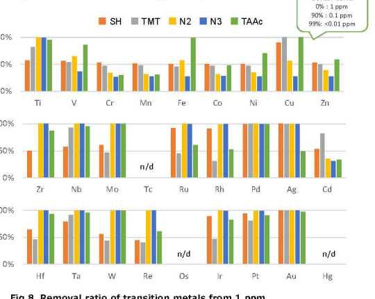
Fig 8. Removal ratio of transition metals from 1 ppm 4 mL ICP-MS standard 1 ppm of each element in 0.5% HNO 3 was flowed in a cartridge (210 mg bed) by ca. 3 mL/min. Concentrations of elements were analyzed by ICP-AES. The detection limit < 2-10 ppb depending on the metals. For Ru, Rh, Pd, Ir, Pt, Au, and Hf, the solution was in 1% HCl.
